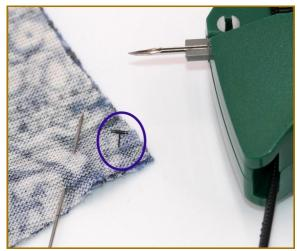
The Microstitch Basting Gun is a very handy addition to your sewing tools. Perfect for keeping corners and seams in place. Extremely helpful when work ing with unruly knits.
