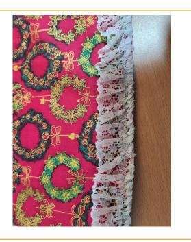
Set up for a 4 thread overlock, using the Gathering Foot. Stitch length 4 and Differential Feed 2. Place the lace under the foot, right side up, and the fabrics through the foot, right side down. Gather the lace onto the fabrics.
