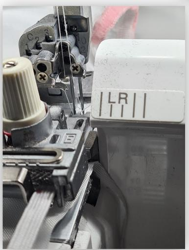
Allow the blade to cut a little sliver off. This makes it easier for you to see what is going on, and not lose the fabric under the foot.
