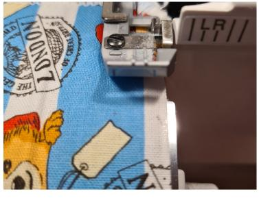
When the needle reaches a few mm from the edge, stop with the needle down. Raise the foot, and pivot the fabric by 90 degrees..
