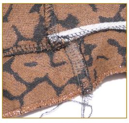
Snip the seam line up to the chain stitch line, and press in opposite directions.
