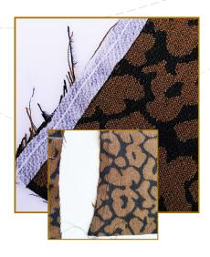
You can use the DF on your overlocker to control the fabric and stop it from stretching.
