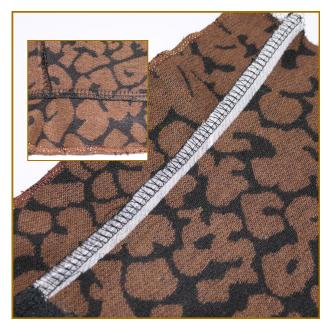
Press seam allowance towards the facing, understitch using a chain stitch. This will prevent the facing rolling outwards.
