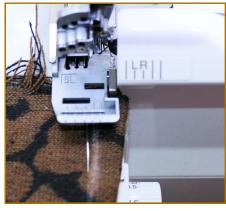
Line the chalk line with the left needle marking on the foot. A 4 thread OL is used, it is stronger than a 3 thread.
