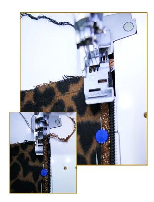
Set your machine up for cover stitch, the triple cover stitch has been used for this skirt. This is to attach the zip the skirt.
